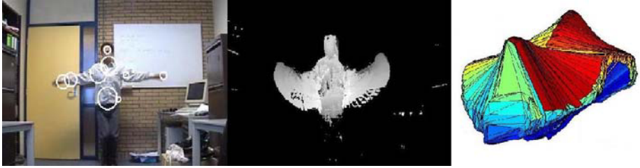
Fig. 5. Human body gesture recognition based on (left to right): spatio-temporal salient points, motion history (i.e., when and where motion occurred), and spatio-temporal shapes [53]
