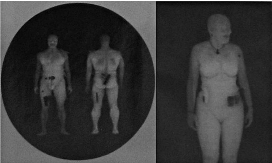
Fig. 9. The three-dimensional holographic imaging systems can detect contraband beneath clothing, yet they raise privacy concerns due to the detailed human figure that is revealed
